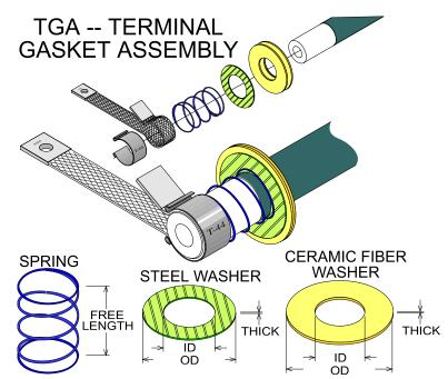
Note: The strap and clamp are shown for illustrative purposes and are not supplied with the TGA assembly.
