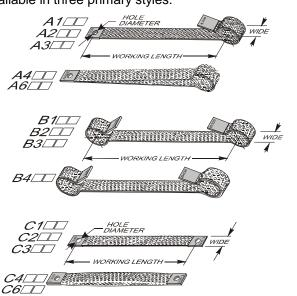
**IDENTIFICATION:** Aluminum straps are stamped with the part number for easy identification and proper matching to the correct diameter Starbars.
